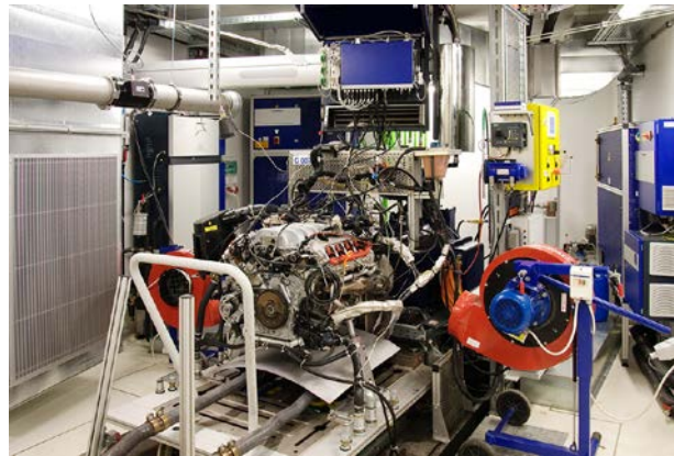
Figure 11. The full functional engine dynamometer
