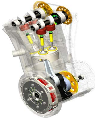
Figure 10. The engine designed and built by the Formula Student team at Széchenyi István University. The engine is 500cc, single cylinder, optimized for formula student race cars.
